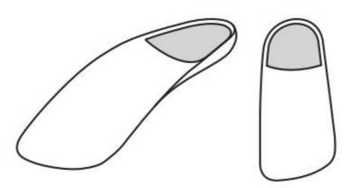
3mm poron added to the heel area of the shell.
